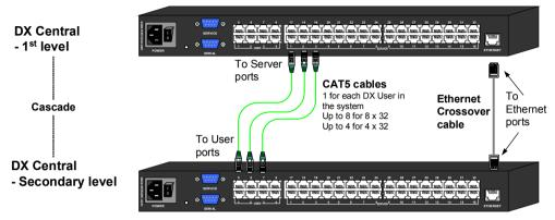
Figure 16 Cascaded DX Central units connected with a Crossover cable
